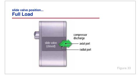
At full load, the slide valve is closed. The compressor pumps its maximum volume of refrigerant, discharging it through both the radial and axial ports.
